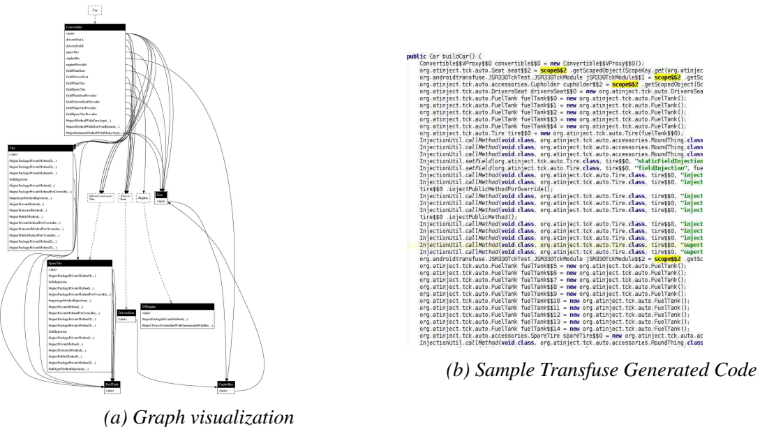
Figure 4.3: Example JSR330 injection graph. This graph contains 8 classes and 66 injection points. Transfuse builds this graph through 382 lines of injection graph code.
